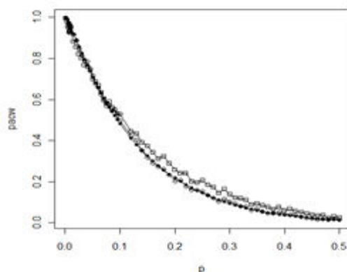
**Figure 4:** Comparison of OC-curves,  $P_{ac}(p)$ ,  $p \in [0; 1]$  — range of non-conforming proportion — between Weibull ( $\theta = 1$ ) (simulated values) and Gaussian case,  $n = 5$ :
