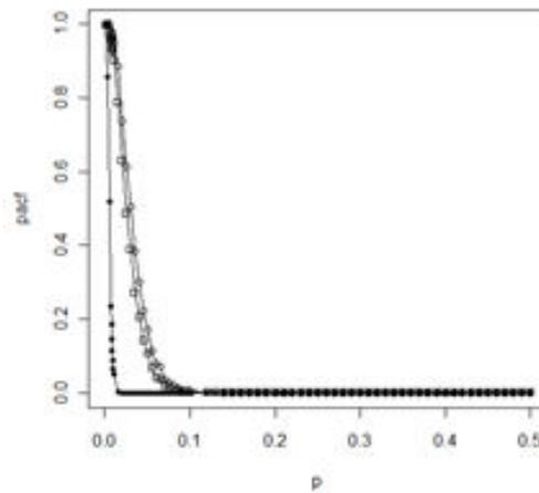
**Figure 6:** Comparison of OC-curves,  $P_{ac}(p)$ ,  $p \in [0; 1]$  — range of non-conforming proportion — between Fréchet ( $\theta = 1$ ) (simulated values) and Gaussian case,  $n = 5$ :
