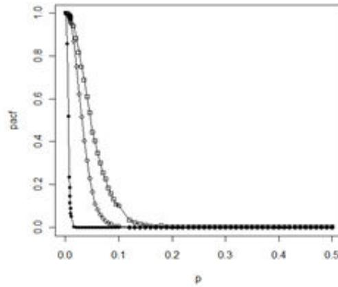
**Figure 5:** Comparison of OC-curves,  $P_{ac}(p)$ ,  $p \in [0; 1]$  — range of non-conforming proportion — between Fréchet ( $\theta = 1$ ) (simulated values) and Gaussian case,  $n = 5$ :
