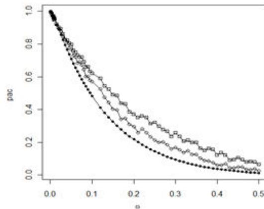
**Figure 2:** Comparison of OC-curves,  $P_{ac}(p)$ ,  $p \in [0; 1]$  — range of non-conforming proportion — between Weibull (simulated values) and Gaussian case,  $n = 5$ :
