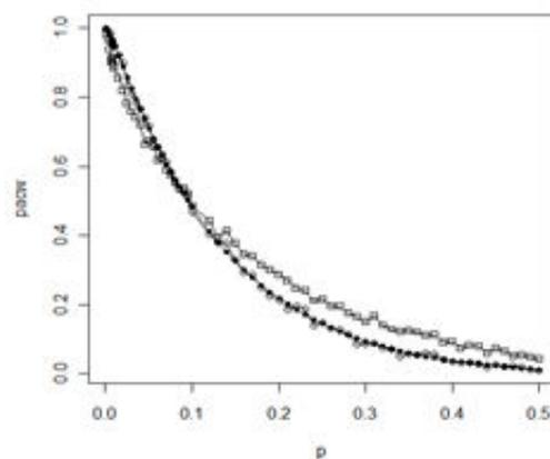
**Figure 3:** Comparison of OC-curves,  $P_{ac}(p)$ ,  $p \in [0; 1]$  — range of non-conforming proportion — between Weibull ( $\theta = 1$ ) (simulated values) and Gaussian case,  $n = 5$ :
