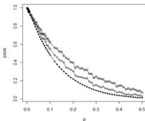
**Figure 1:** Comparison of  $OC$ -curves,  $P_{ac}(p)$ ,  $p \in [0; 1]$  — range of non-conforming proportion — between Weibull (simulated values) and Gaussian case,  $n = 5$ :
