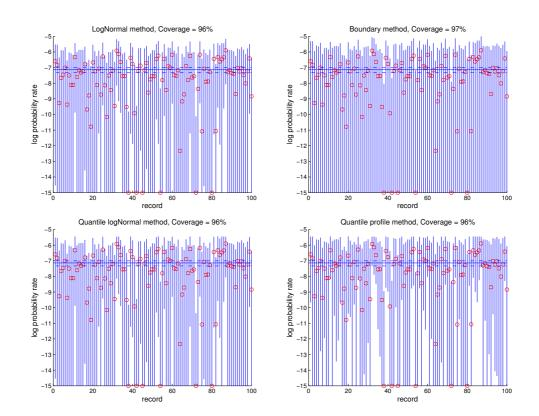
Figure 7: Confidence intervals for 100 records of the length of 100 hours. Roll series for 45° heading and with critical roll angle of 60°. Top left: lognormal method. Top right: boundary method. Bottom left: quantile-lognormal method. Bottom right: quantile-profile method.
