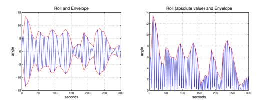
Figure 5: The roll angle series with envelope for 5 minutes. Left: original roll series. Right: roll series in absolute value.
