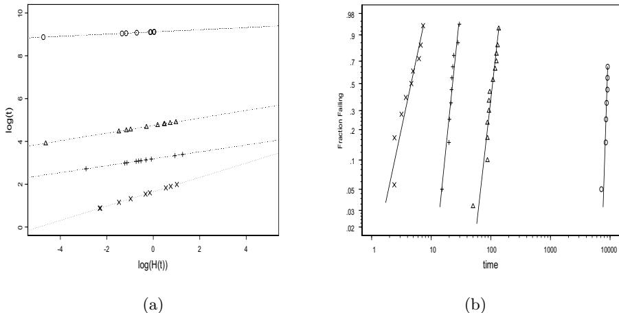
**Figure 1:** Weibull fit for PET film data, Table 1.
